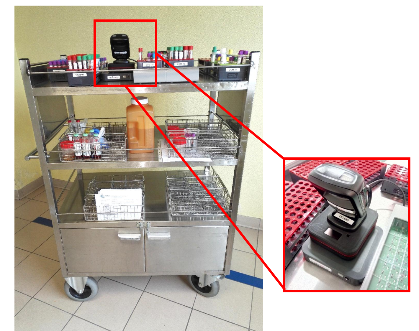
Figure 1. Mini Indexor System. Connected to the Hospital wireless network, all sample barcodes were read prior to transport to the Laboratory.
